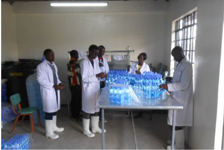
Fountain Valley water team at the water production house packaging, labelling and sealing the mineral water.
